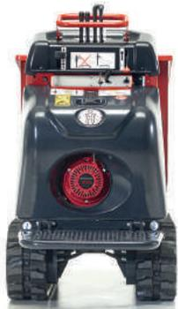
◀ It is a very compact machine at 758 mm width which allows it to pass through narrow spaces such as doors and gates.
